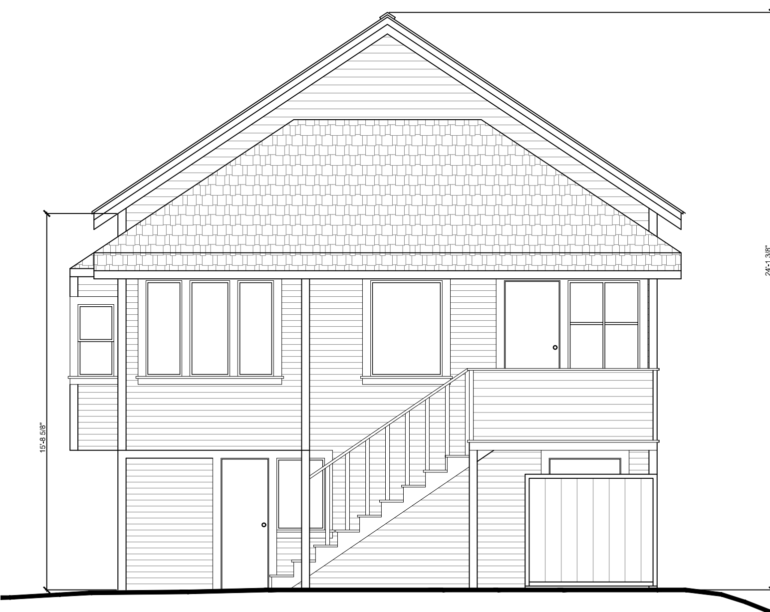
5 EXISTING EAST ELEVATION SCALE 1/4" = 1'-0"
