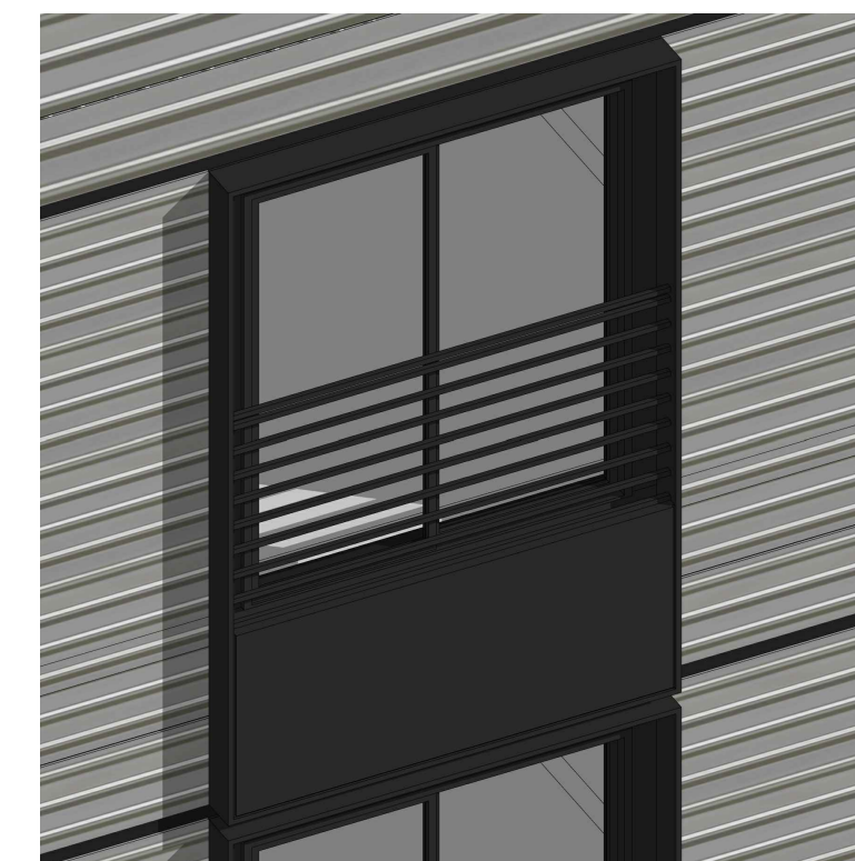
C. TYPE 3 : VINYL WINDOWS * FLUSH MOUNTED SLIDER WINDOW WINDOW FIN/TRIM BLACK OR EQUAL
