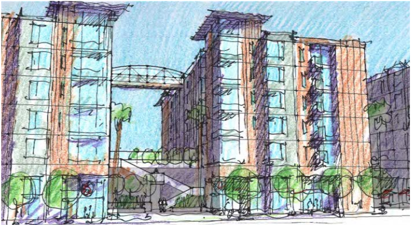
Looking East across San Pablo Boulevard: Podium access stair and roof deck bridge connect the north and south halves of the project.
